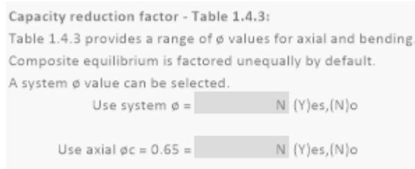
The default factors are set to  $\phi=0.8$  for concrete, and  $\phi=0.9$  for steel as per table 1.4.3y. The options provided allow the user to set an overall system  $\phi$  or set the concrete factor to  $\phi=0.65$  (being axial).
